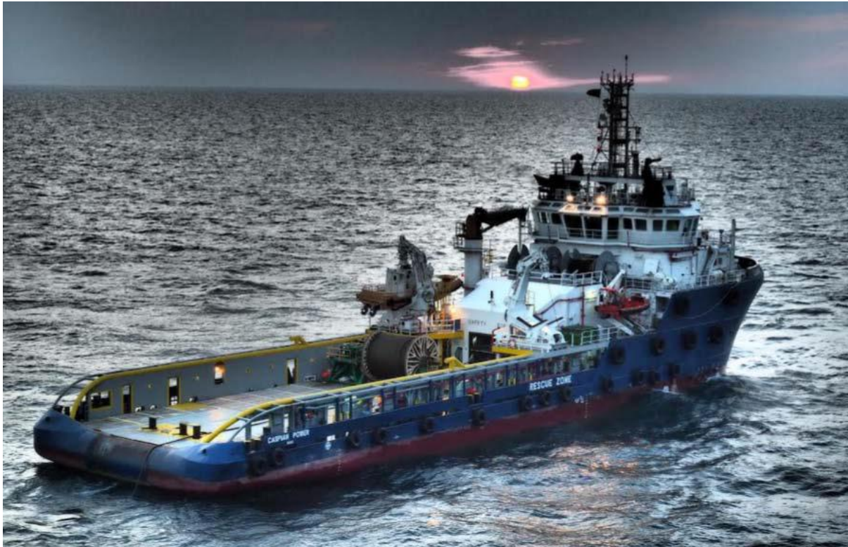
AHT CASPIAN POWER in the process of spooling new mooring wire onto drilling rig "ISTIGLAL" Shah Deniz A - Caspian Sea. Photo : BP Marine rep. Pieter C Holtes © (o/b of drilling rig "Istiglal")
